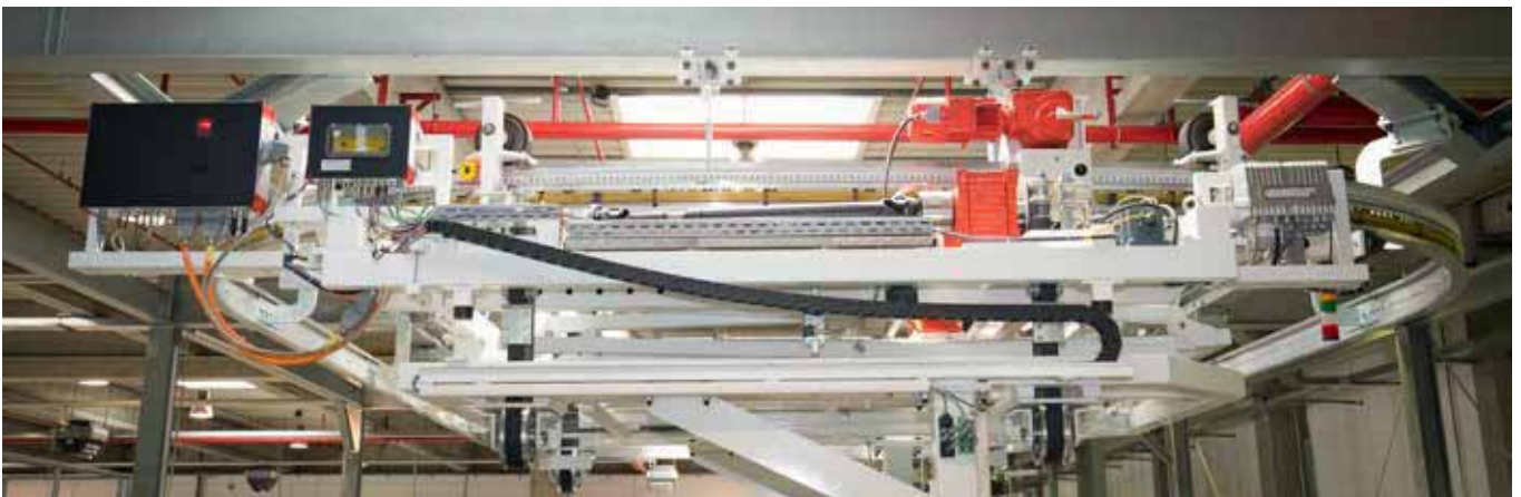
Safety electrified monorail system (EMS Safety)
